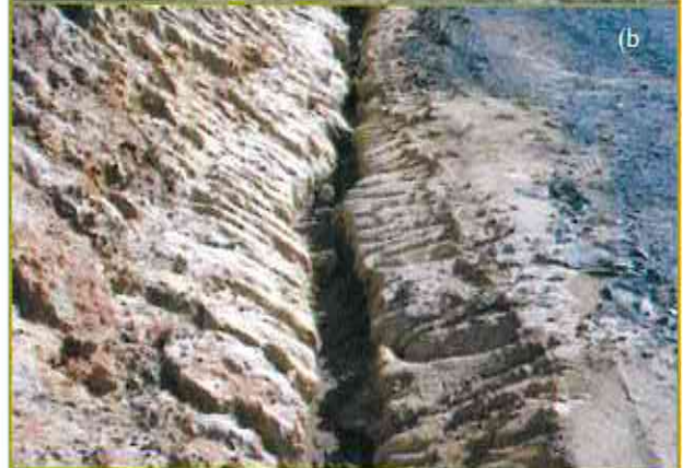
Figure 6 (a). Tunnel erosion resulting from construction of a culvert in dispersive clay (b). Tunnel erosion caused by installation of optical fibre cable in dispersive soil.
