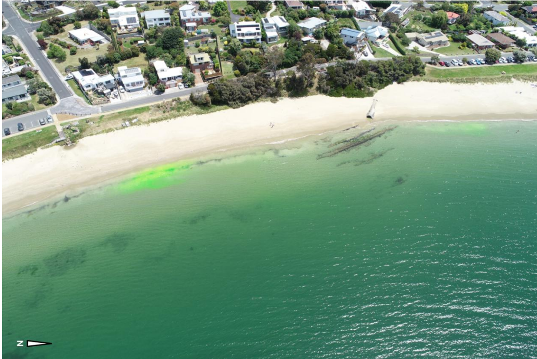
Figure 10. Non nadir aerial image of fluorescent dye discharging from Mid Beach and Illawarra outfalls in the incoming tide .
