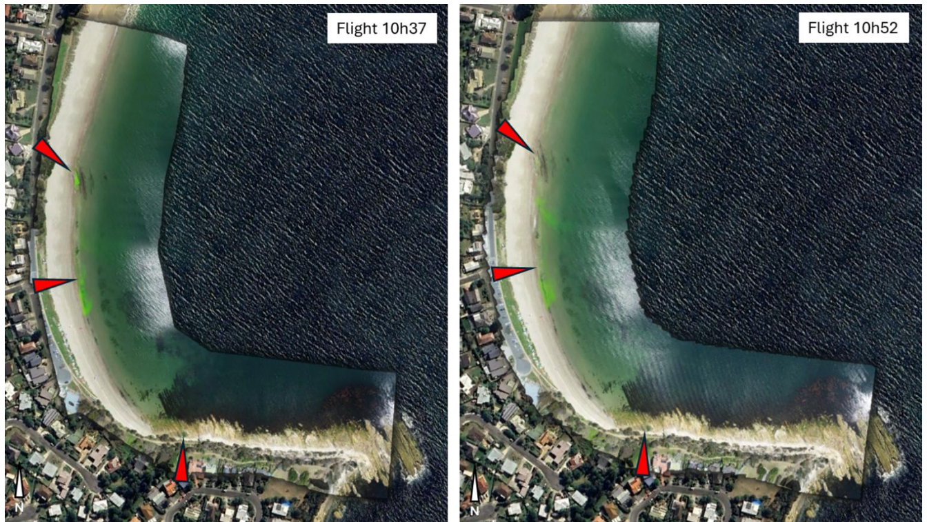
Figure 7. Orthomosaic of aerial images showing fluorescent dye discharging from the three southern Blackmans Bay outfalls (marked with red arrows) into low tide (background map: Google Earth Pro).
