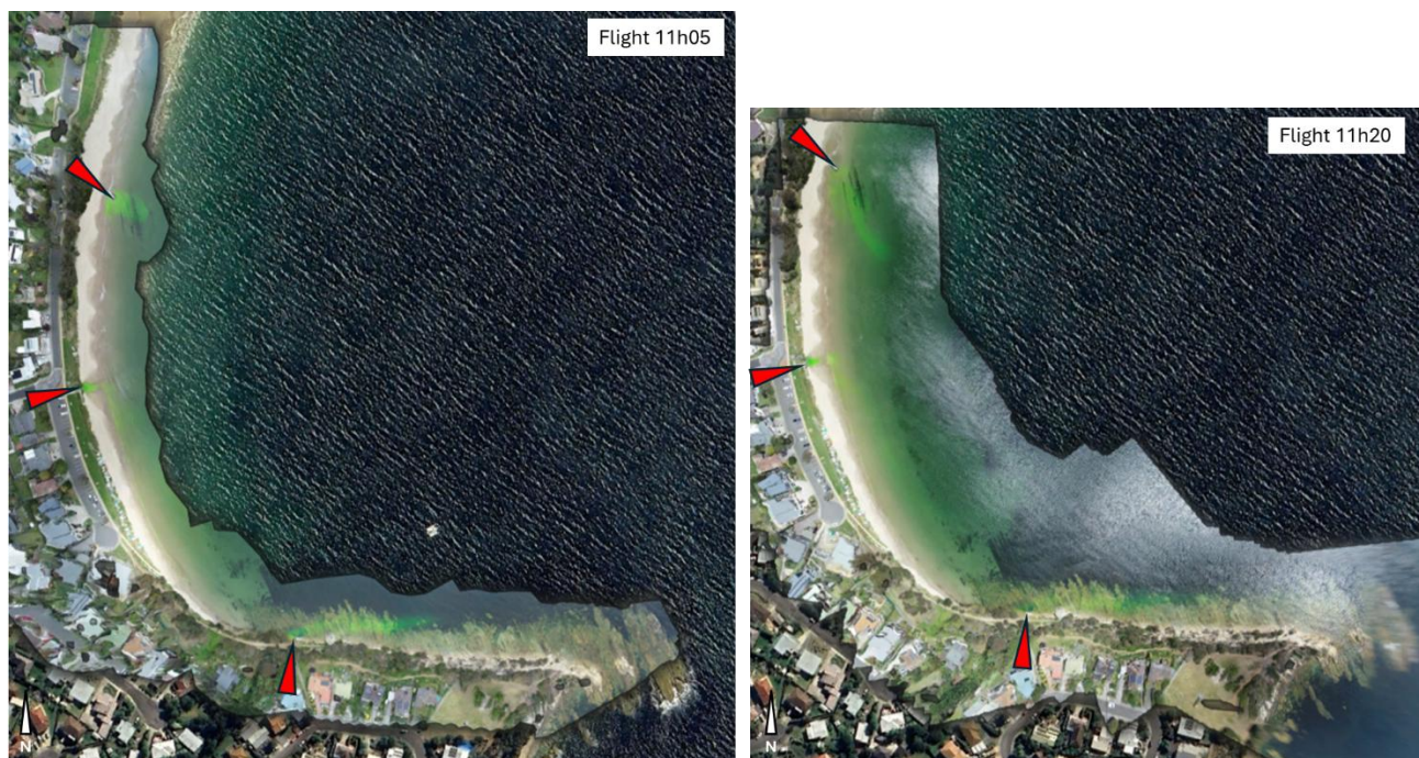
Figure 4. Orthomosaic of aerial images showing fluorescent dye discharging from the three southern Blackmans Bay outfalls (marked with red arrows) in the high-outgoing tide (background map: Google Earth Pro).
