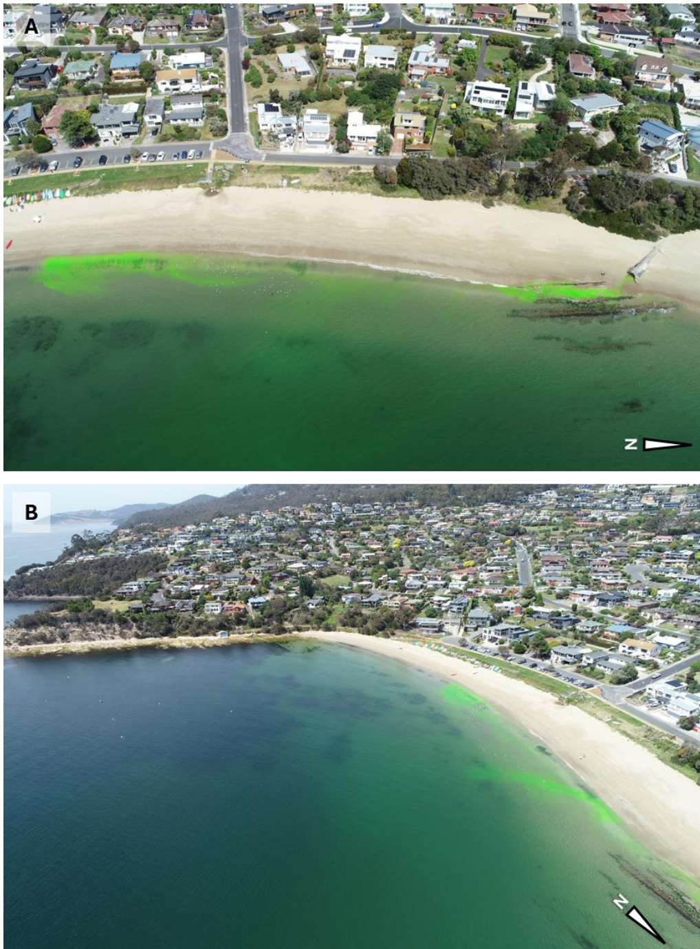
Figure 8. Non nadir aerial images of fluorescent dye discharging from (A) Mid Beach and Illawarra, and (B) all three stormwater outfalls in the low tide .
