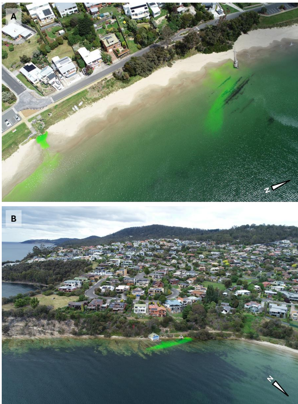
Figure 5. Non nadir aerial images of fluorescent dye discharging from (A) Mid Beach and Illawarra, and (B) Flowerpot stormwater outfalls in the high-outgoing tide .
