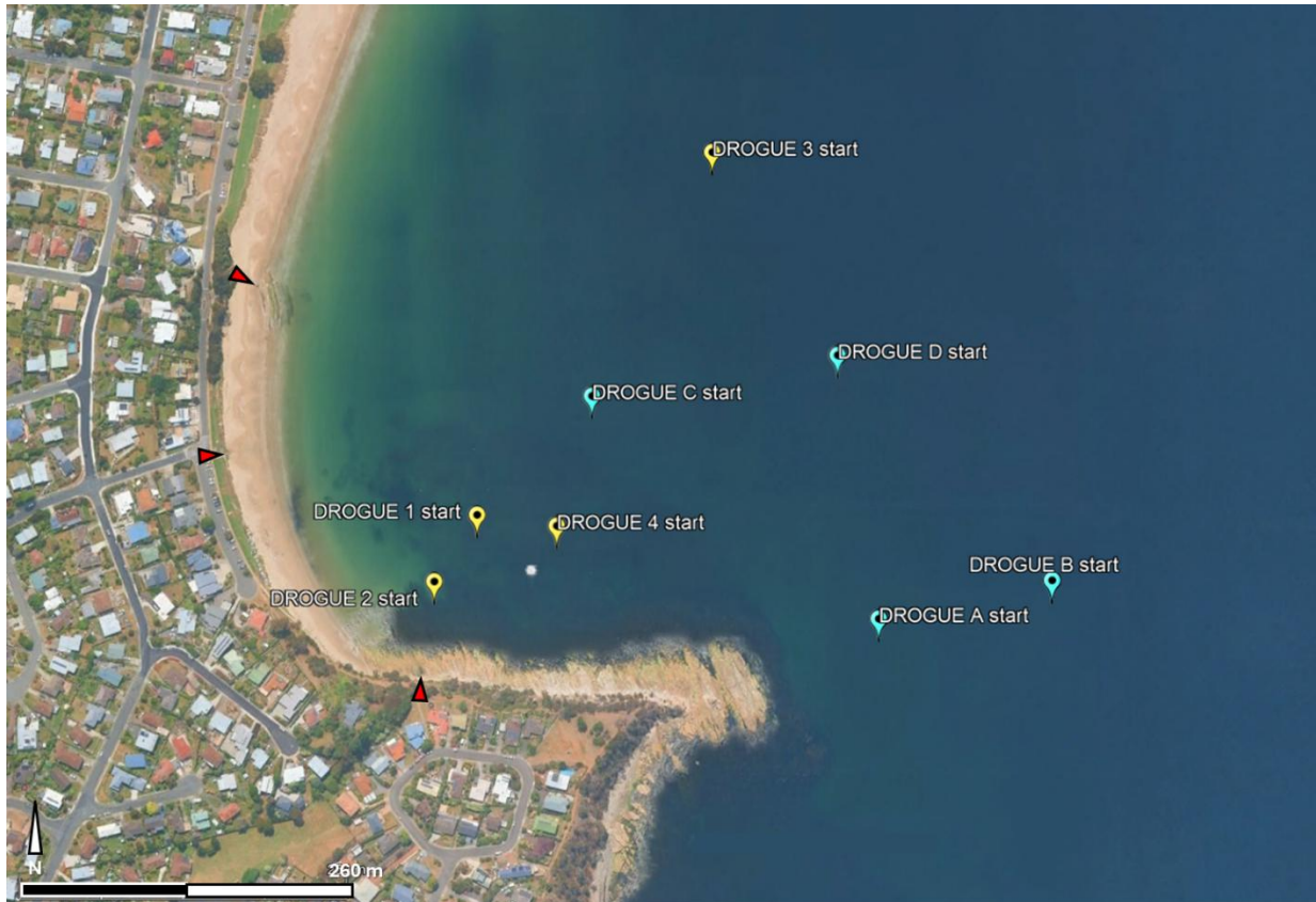
Figure 12. Starting locations of the two different types of drogues deployed in south Blackmans Bay, relative to the three stormwater outfalls in the area (locations marked with red triangles). Deeper water drogues A – D (blue markers) and shallow water drogues 1 – 4 (yellow markers).
