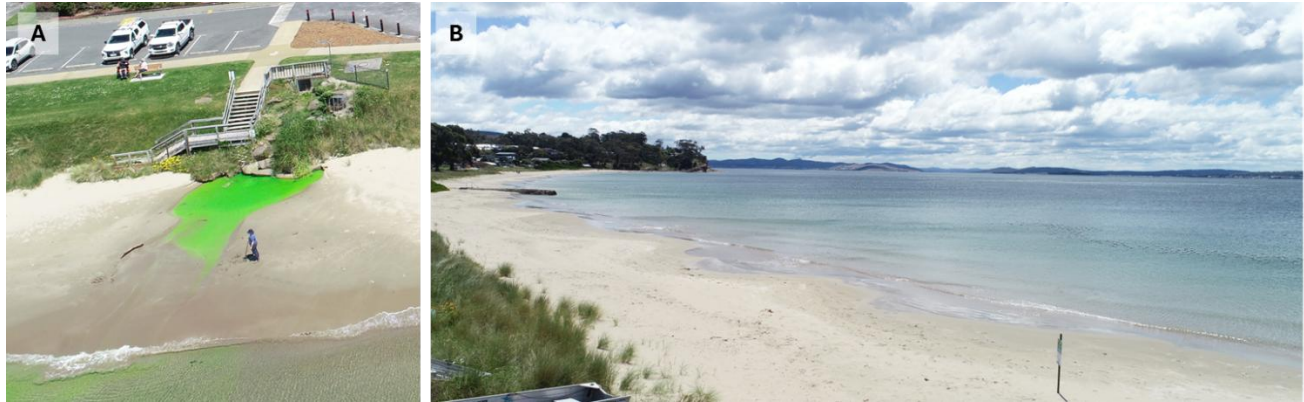
Figure 6. One hour after dye dosing, (A) the tide had dropped so that the Illawarra stormwater outfall was no longer discharging to the bay, and (B) the dye-dosed effluent from Mid Beach outfall had dispersed and was no longer visible.
