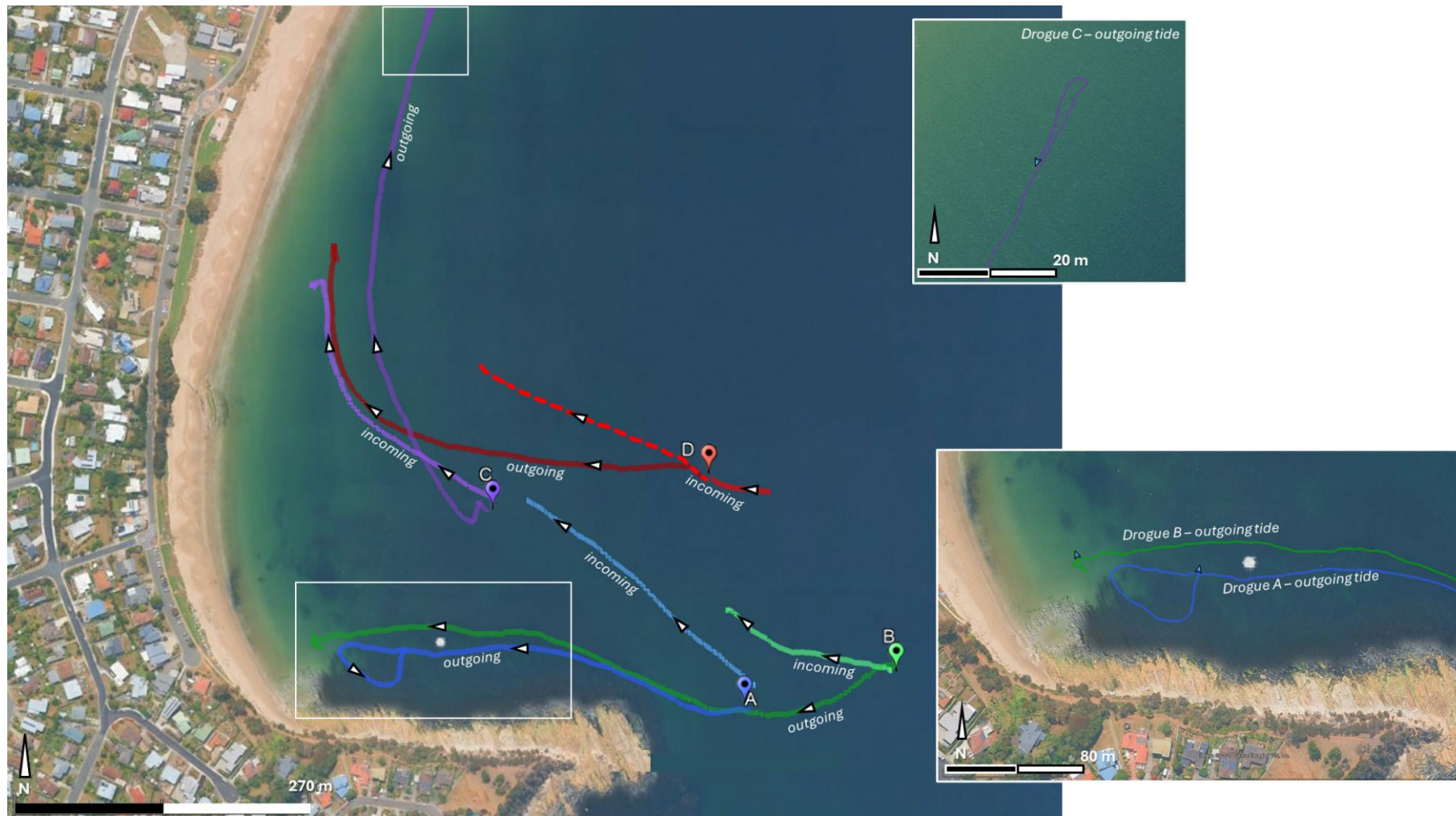
Figure 13. Track logs for four deeper water drogue deployments, from starting points A – D in the outgoing and incoming tide. Drogues were returned to the same starting point for both tides. White arrows show direction of drogue movement, inserts show detail of drogue movement at the end of outgoing tide deployment. Dashed line for drogue D in the incoming tide indicates presumed track of drogue to the recorded end point location (flat battery, track not fully recorded).
