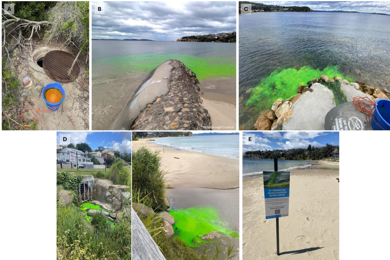
Figure 2. Fluorescein dye dosing into the three southern Blackmans Bay stormwater outfalls at high tide on 8 December 2025. (A) Dosing at sump on Mid Beach outfall, (B) dyed effluent discharging from the Mid Beach outfall (C) dosing directly into the discharging Flowerpot outfall, (D) dye-dosed stormwater discharging from Illawarra outfall to the drainage channel on the beach, and (E) Kingborough Council public information signage during the dye study.
