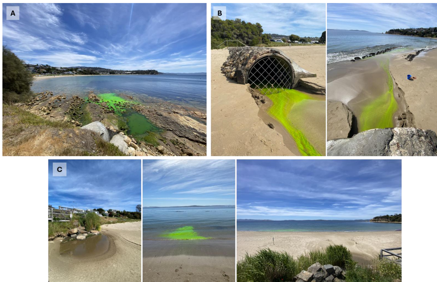
Figure 3. Fluorescein dye dosing into the three southern Blackmans Bay stormwater outfalls at low tide on 12 December 2025. (A) Flowerpot outfall, showing dye in rock pool, (B) dye-dosed stormwater discharging at low volume from Mid Beach outfall, and (C) no stormwater discharge from Illawarra outfall and no drainage channel across the beach, so dye was added directly to water at the shoreline.
