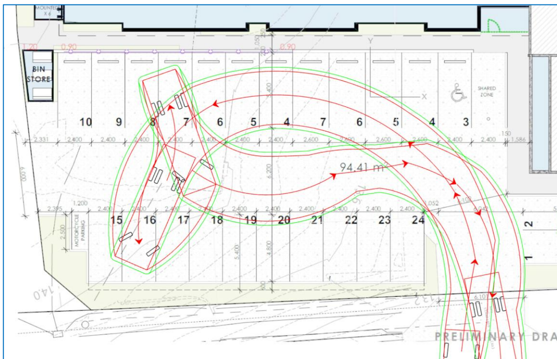
Diagram 7.12 – Swept path of a medium rigid vehicle entering and leaving the site
