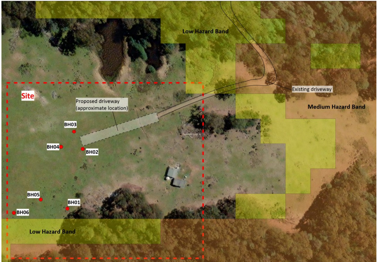
Figure 4 – Bore Hole Locations
