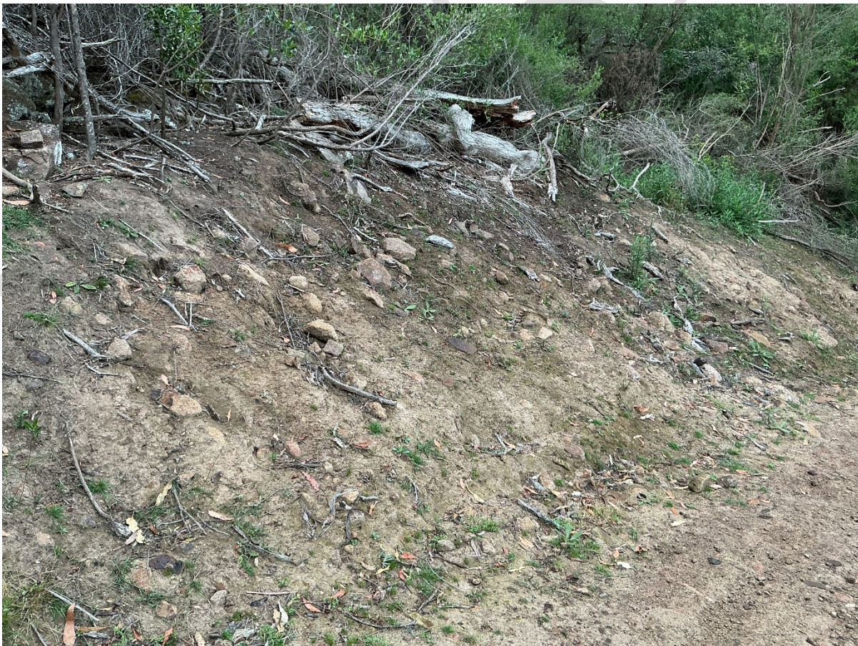
Photo 2 Colluvium deposits in the existing road cut.
