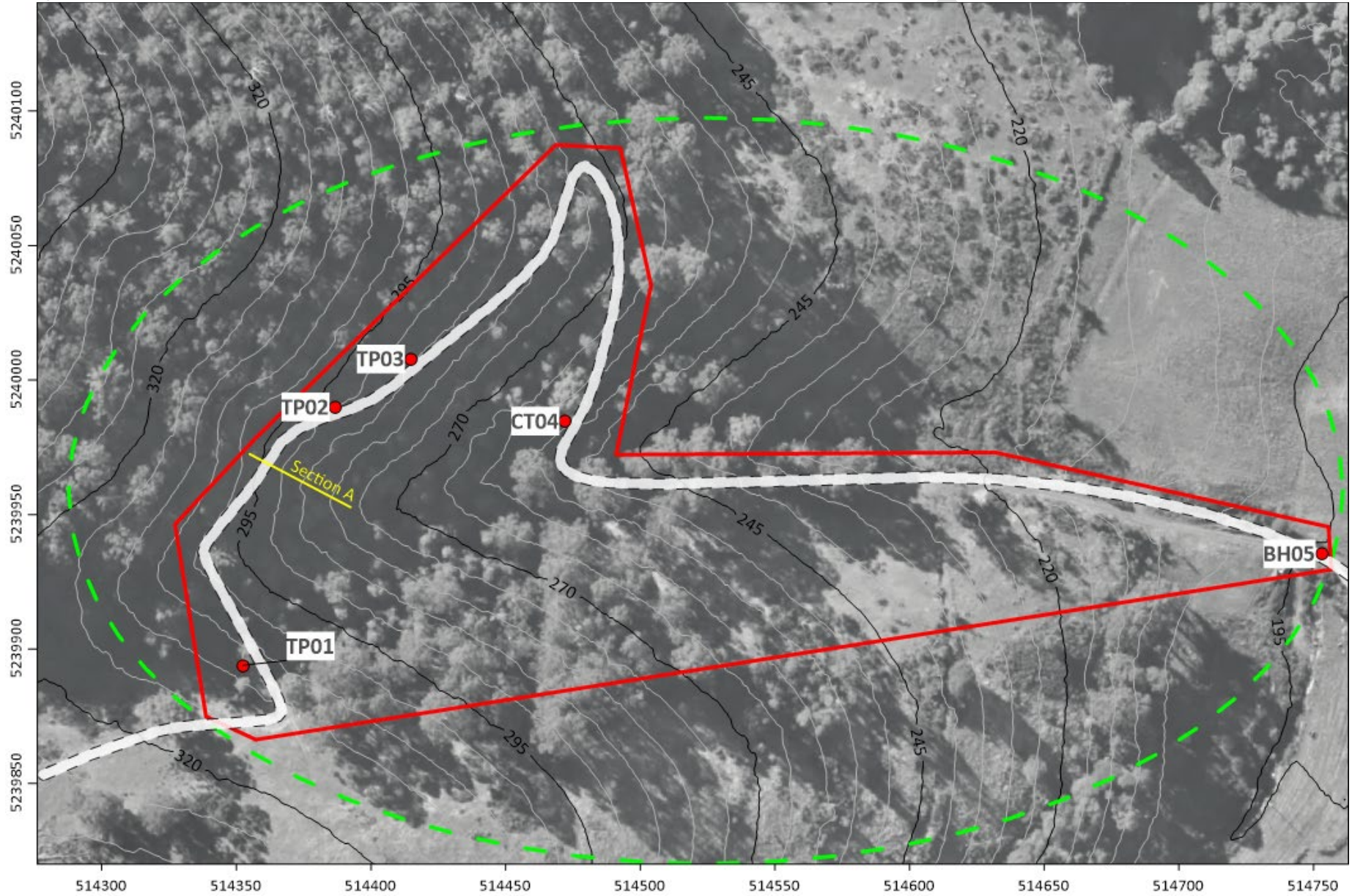
Map 4 Soil testing locations and geotechnical model cross section
