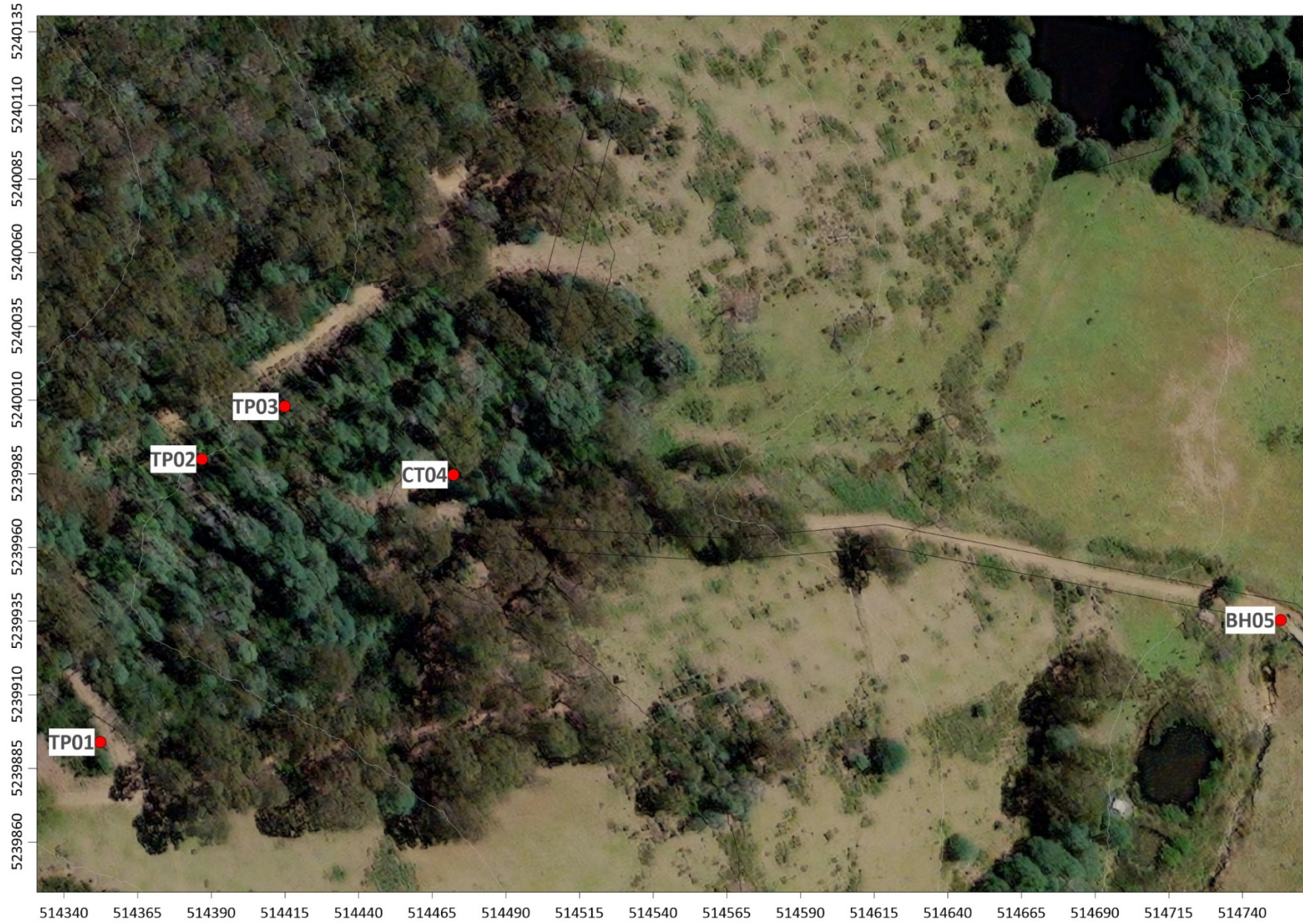
Figure 1 Site Borehole Locations
