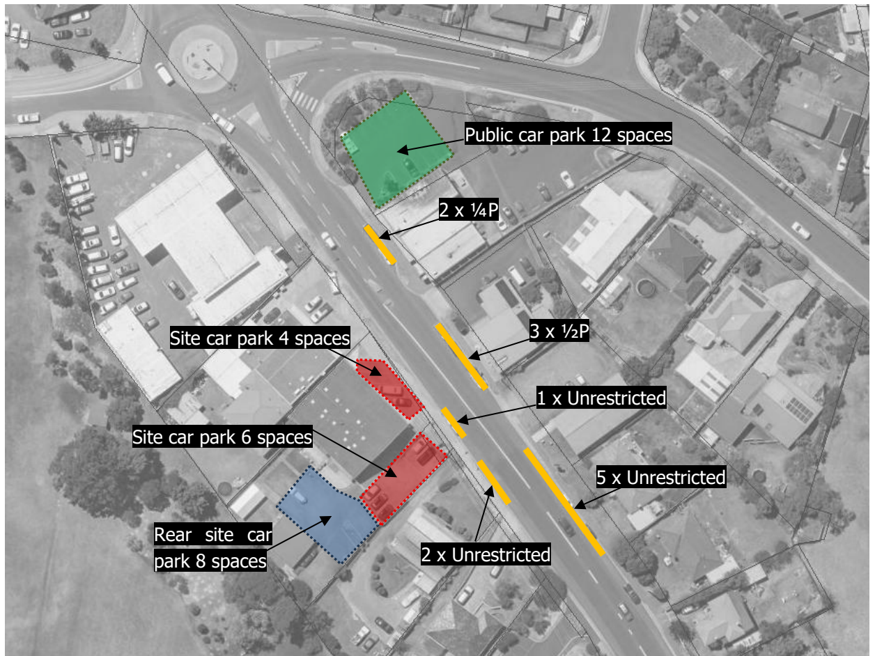
Figure 4 On-Site and Nearby Car Parking
