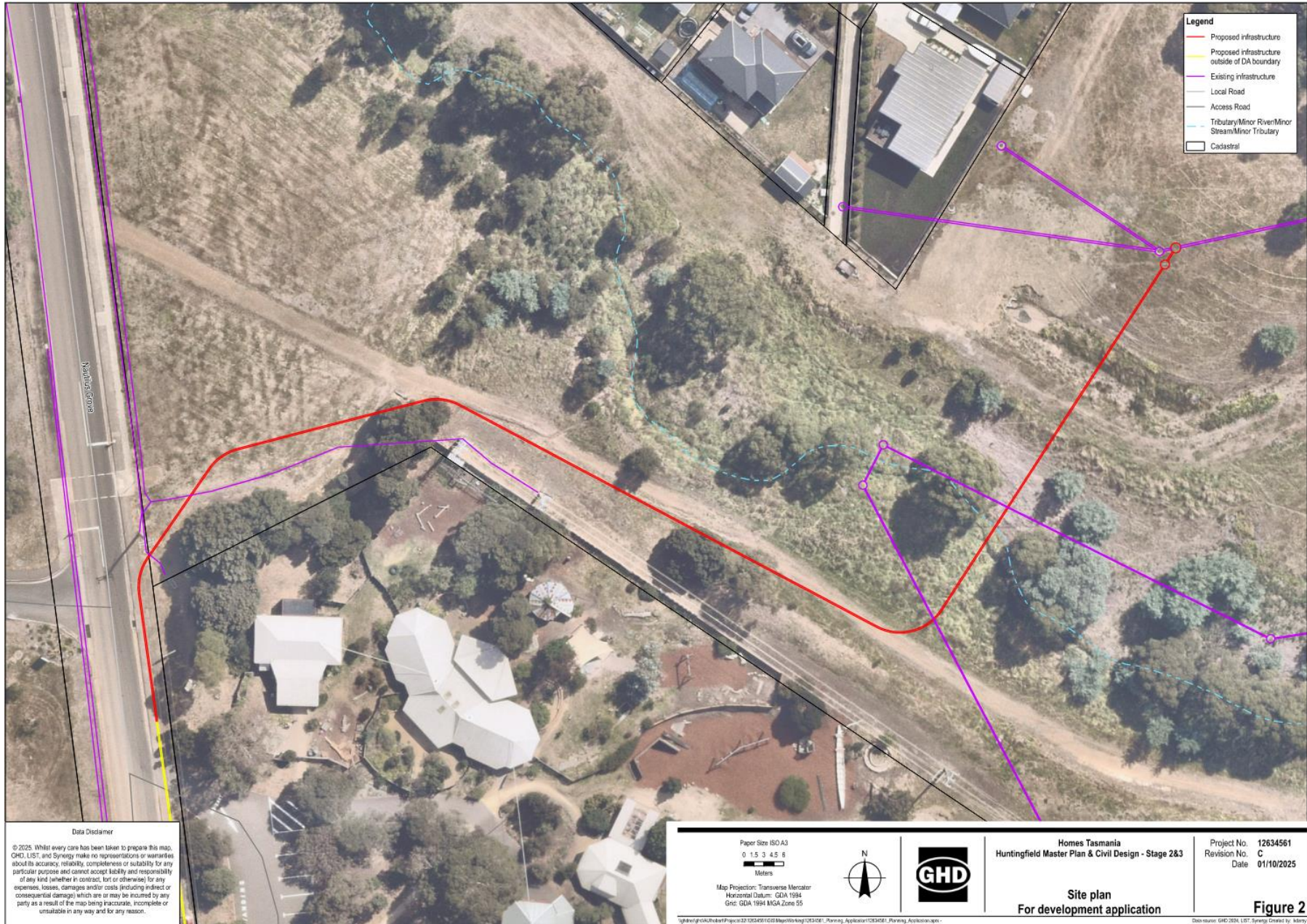
Figure 6 Proposed sewer works shown in red
